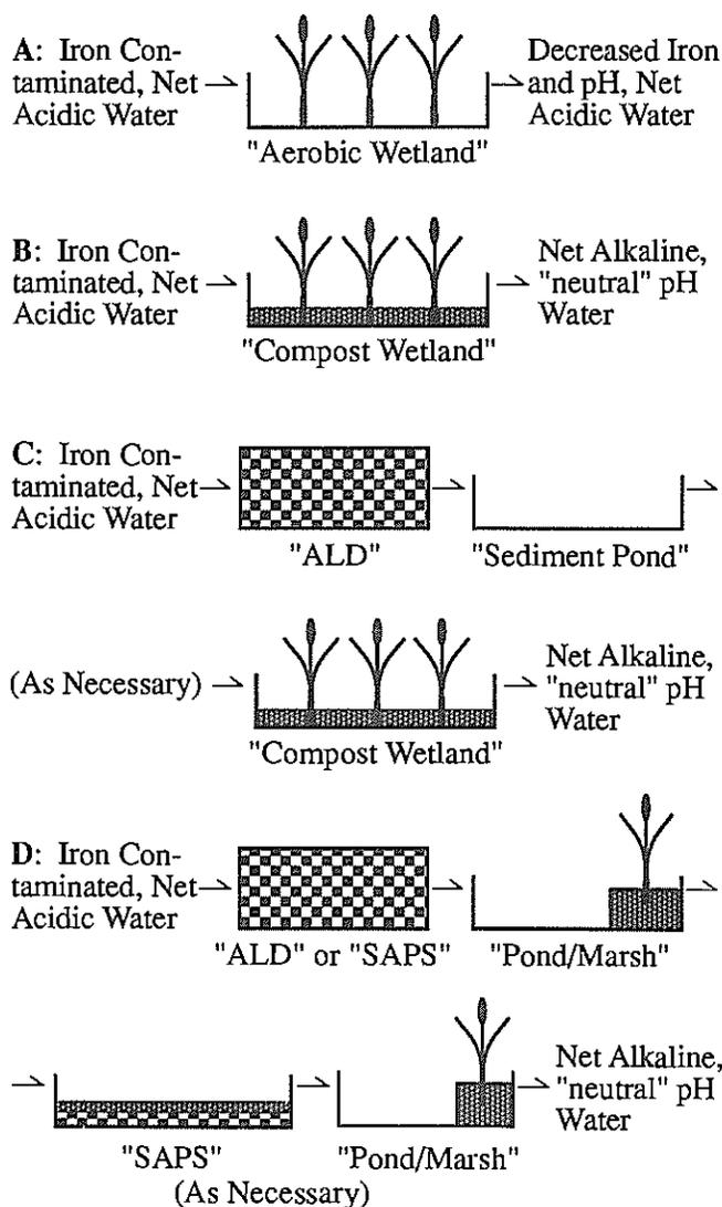
Figure 1. Evolution of passive, wetland treatment technology.
