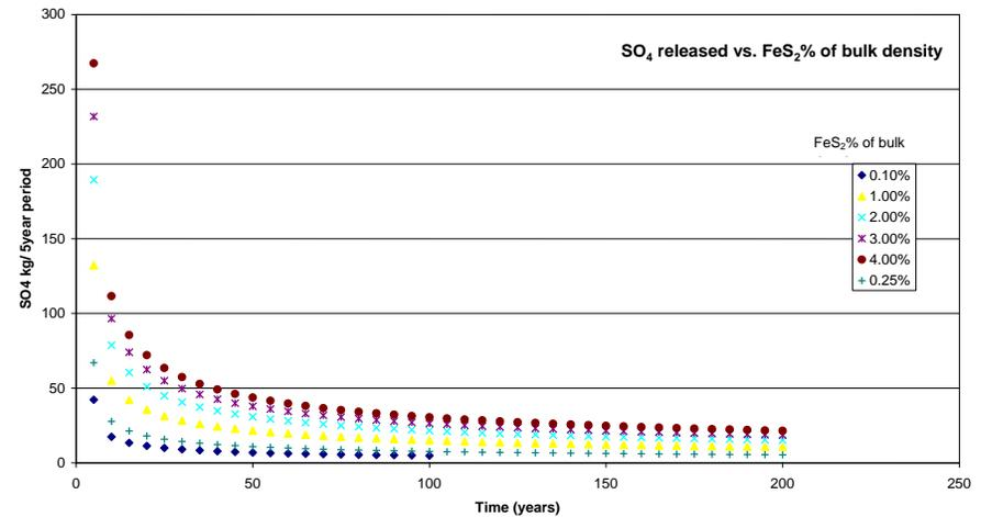
Figure 2: Results of PYROX sensitivity modeling of typical Witwatersrand tailings (incl. sensitivity analysis)sis
