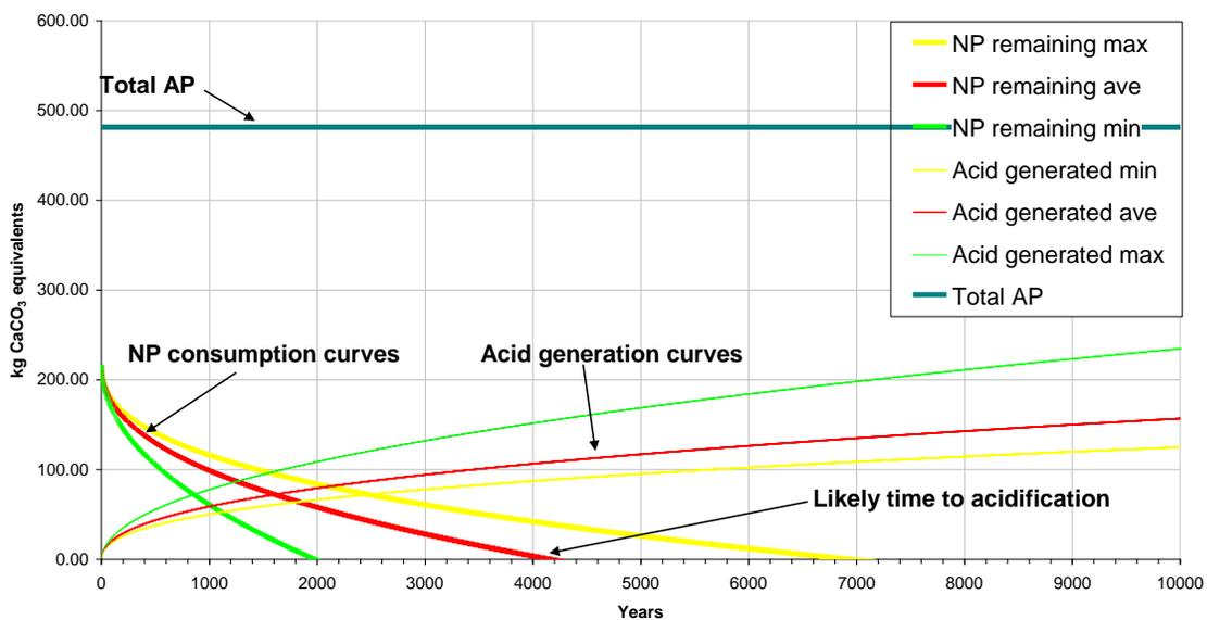
Figure 3: Cumulative curves for consumption of neutralisation capacity and acid generation in typical Witwatersrand FRDs.
