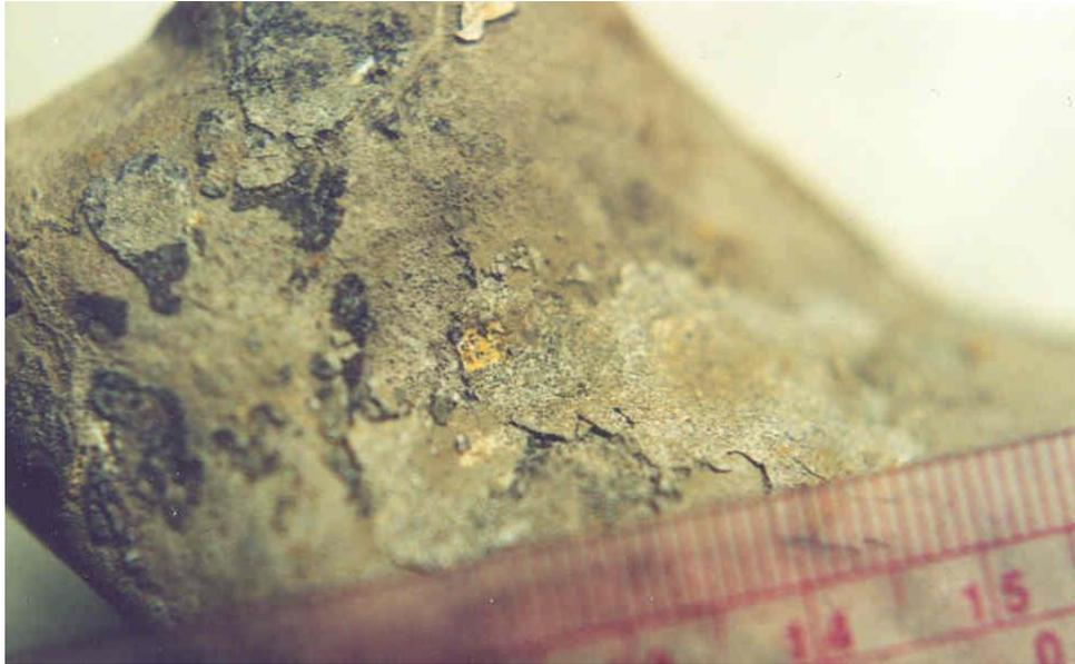
Figure 2A. Photograph of coated limestone fragment from Filson 1 VFP, sample 11. Scale in cm and mm. White coating is Al-rich, black coating is similar to organic matter in other samples. Small scale divisions are millimeters.
