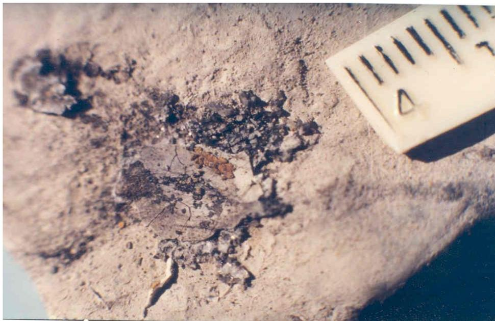
Figure 2B. Photo of patch and associated gypsum crystals (black and white speckled area above patch) on top of limestone. The patch is inferred to be a contact point with another fragment. Scale divisions in millimeters.
