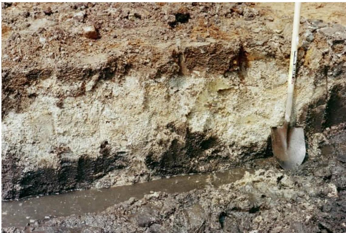
Figure 4. Photo of a trench wall in the Jennings vertical flow pond, showing red Fe oxide zone at top, white Al precipitate in limestone in the middle, and FeS-bearing compost at the bottom.
