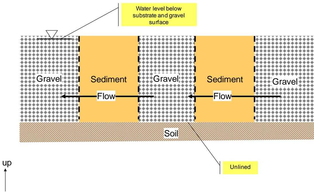
Figure 4. Theoretical layer design; (a) plan view, solid fill is substrate, (b) section view.
