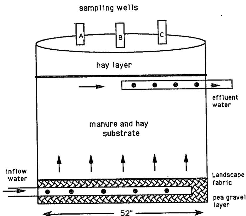
Figure 1: Single Stage reactor constructed of 500 gallon HDP tank and filled with composted cow manure and hay substrate. Wells A, B, and C have sampling levels of 10", 20", and 30" from the base of the substrate.
