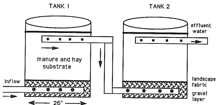
Figure 2: Double Stage reactor constructed of 2 200 gallon HDP tanks filled with composted cow manure and hay substrate. Effluent from TANK 1 discharges directly into tank 2.
