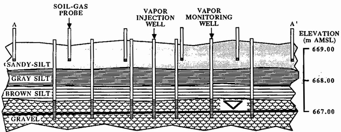
Figure 3. Map view and cross-section of both sampling grids. Vapor injection well and vapor monitoring wells (radial grid) are completed in the unsaturated portion of the gravel unit. Soil-gas probes (rectangular grid) are completed in the red sandy-silt unit.
