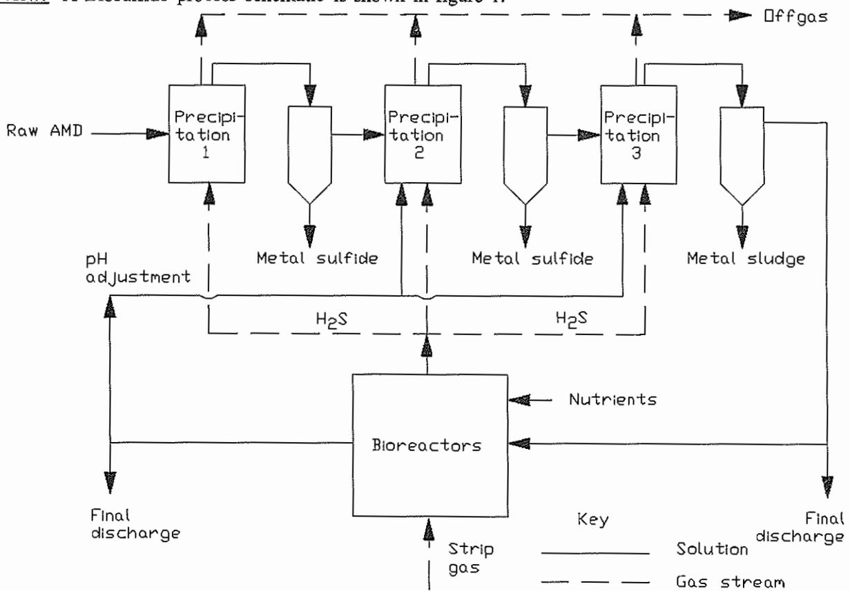
Figure 1. Biosulfide process schematic.
