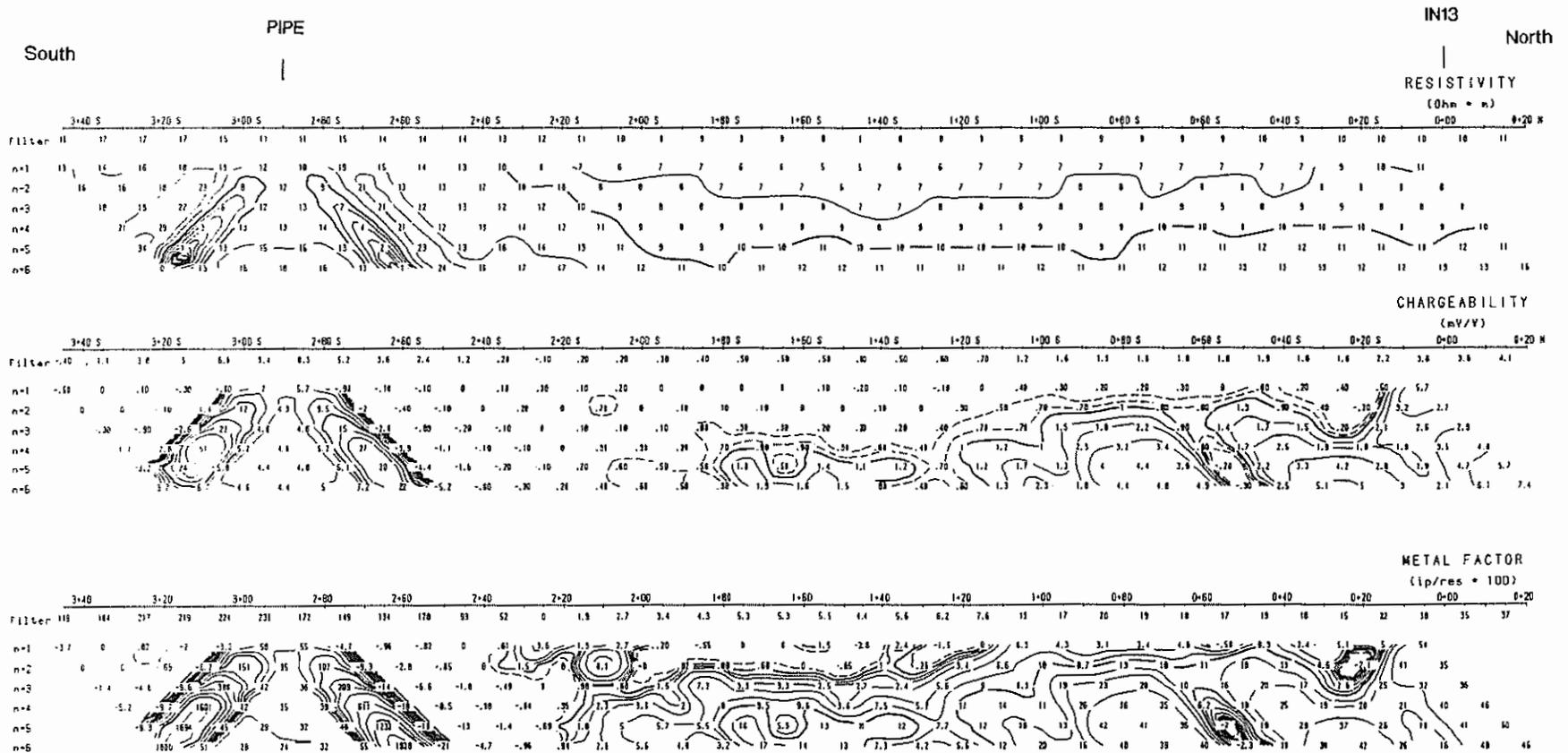
Figure 11. Induced polarization and resistivity data Copper Cliff Tailings.
