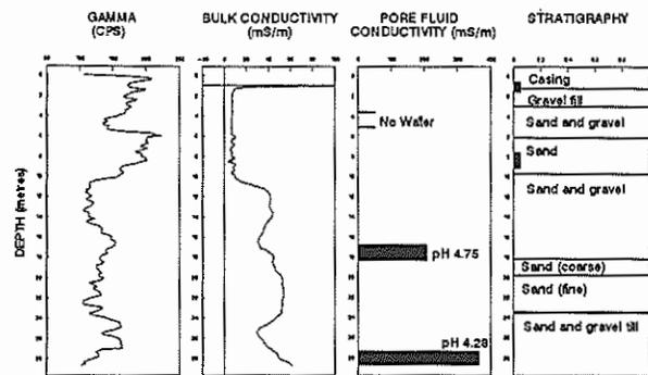
Figure 8. Downhole geophysical logs - Hole T2.
