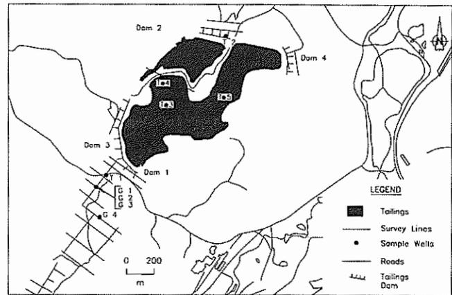
**Figure 4. Levack Tailings - Ground survey lines and sampling well locations.**
