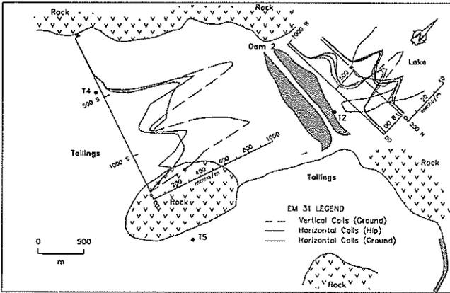
**Figure 5. Levack Tailings North Dam - Shallow ground conductivity data (EM31).**
