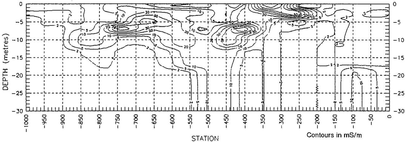
**Figure 7. North Dam Line 00 - Vertical conductivity section.**
