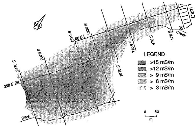
**Figure 6. Levack Tailings South Dam - Deep ground conductivity (EM34, 20 metre coil separation, vertical coils).**
