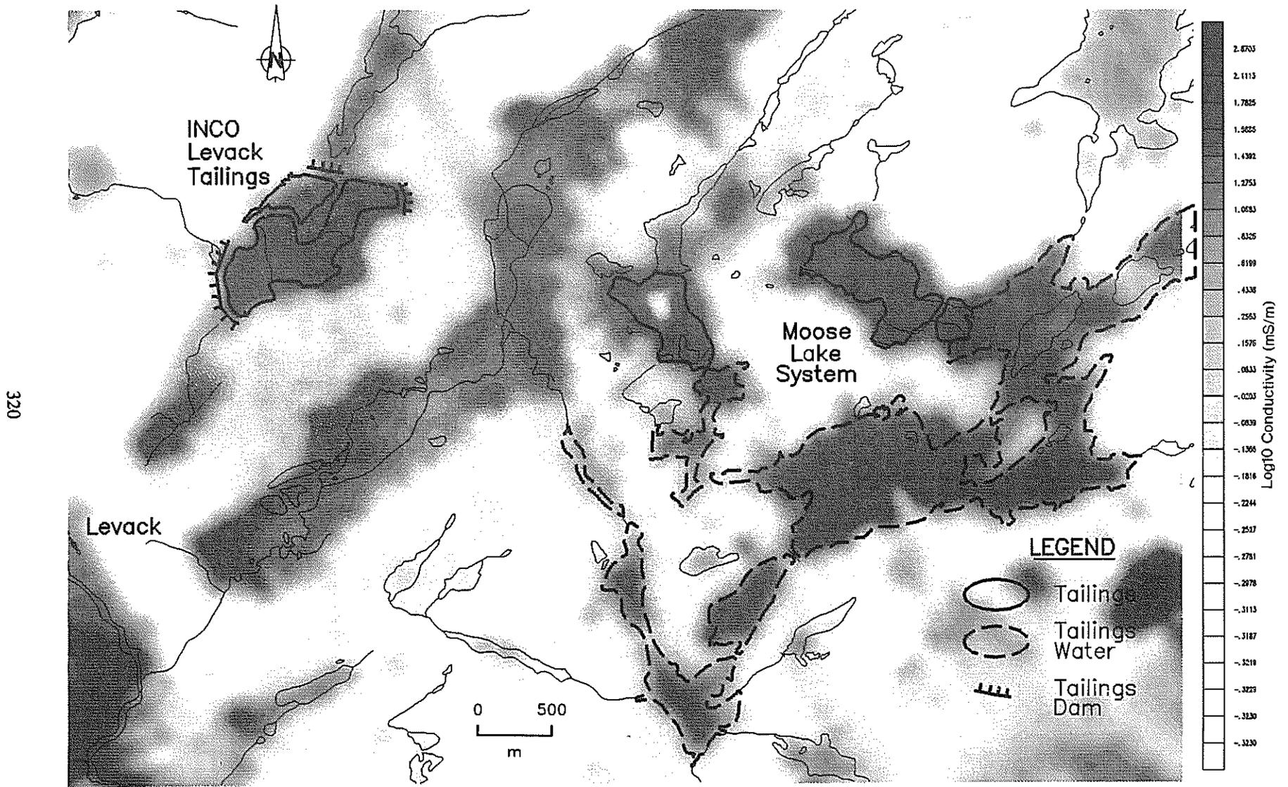
Figure 3. Levack Area - Airborne conductivity data and surface drainage.
