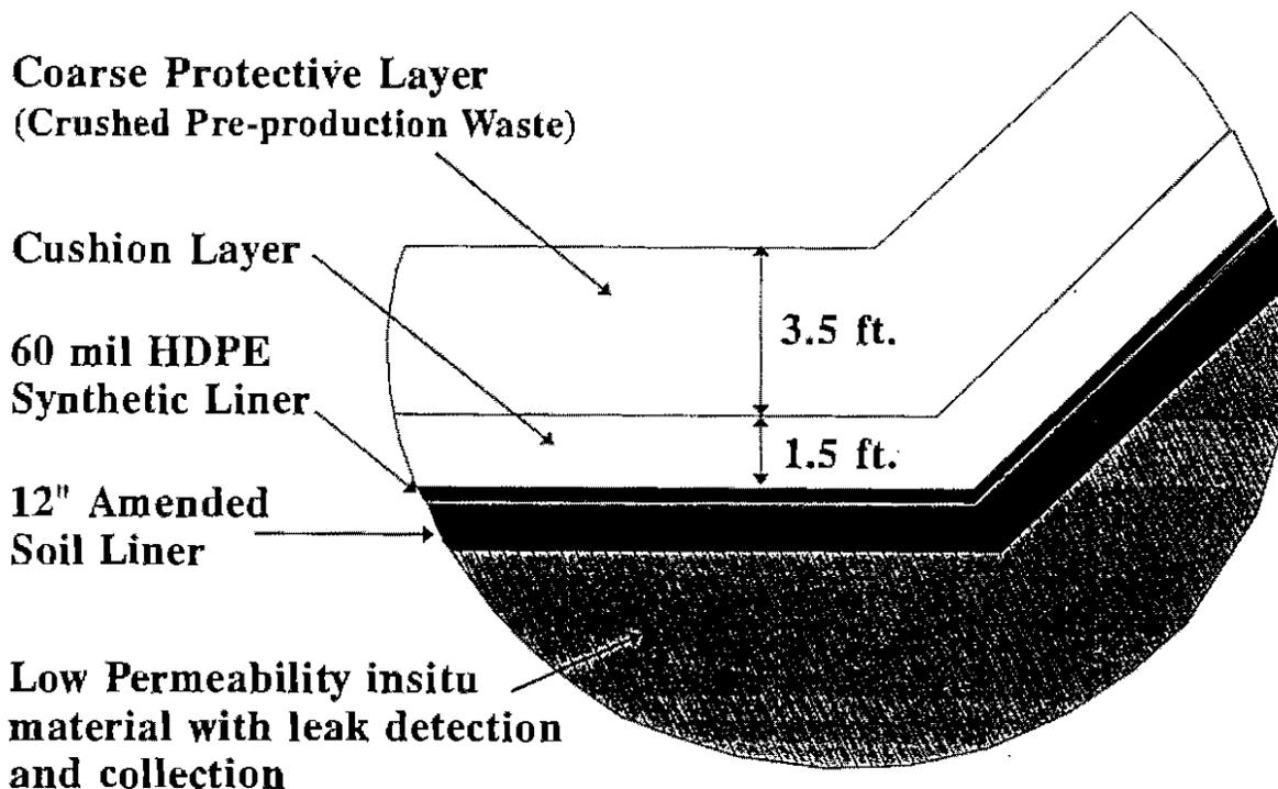
Figure 1. Schematic diagram of the composite liner.
