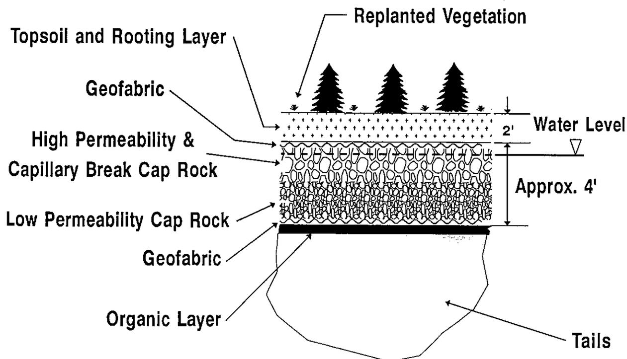
Figure 2. Schematic diagram of the multi-layer reclamation cover.
