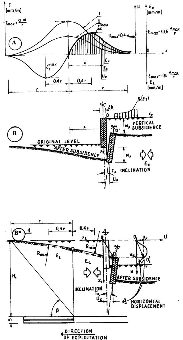
Figure 2. Mine-induced subsoil deformations in the construction's support zone.
