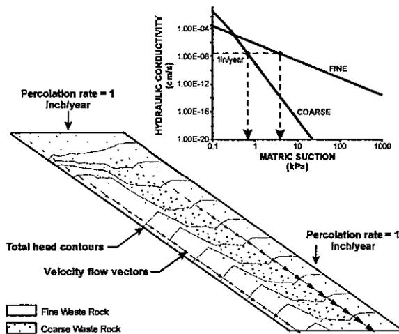
Figure 8. Preferential flow through layered waste rock
