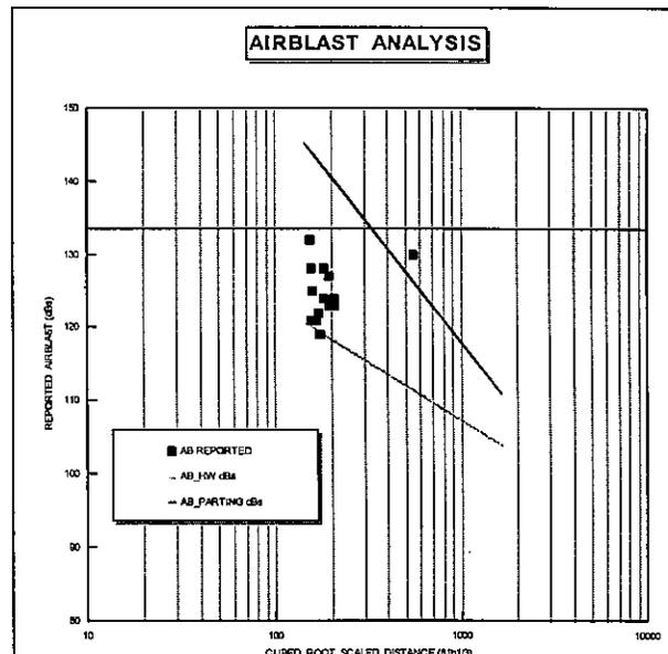
Figure 9 Compliance with airblast limitations.
