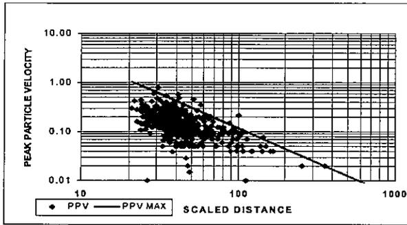
Figure 11 Regression analysis of blasting data.
