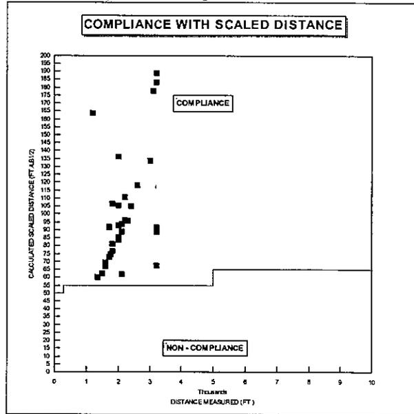
Figure 5 Compliance with scaled distance limitations.
