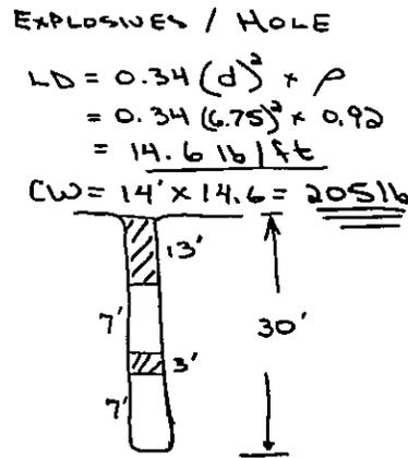
Figure 2 Blast hole cross section.
