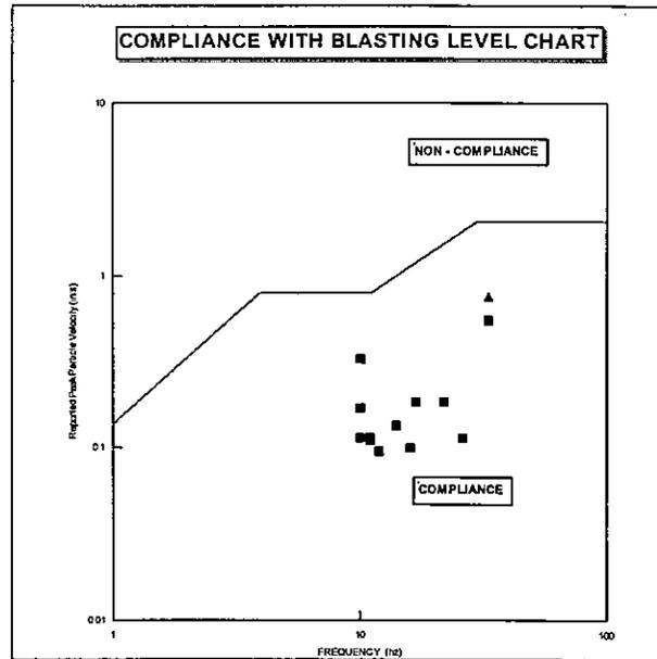
Figure 8 Compliance with blasting Level Chart limitations.
