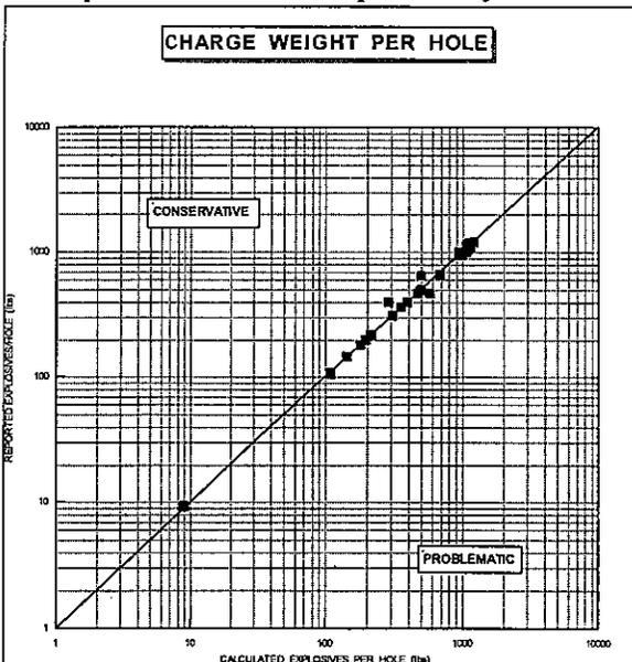
Figure 1 Charge weight per hole.
