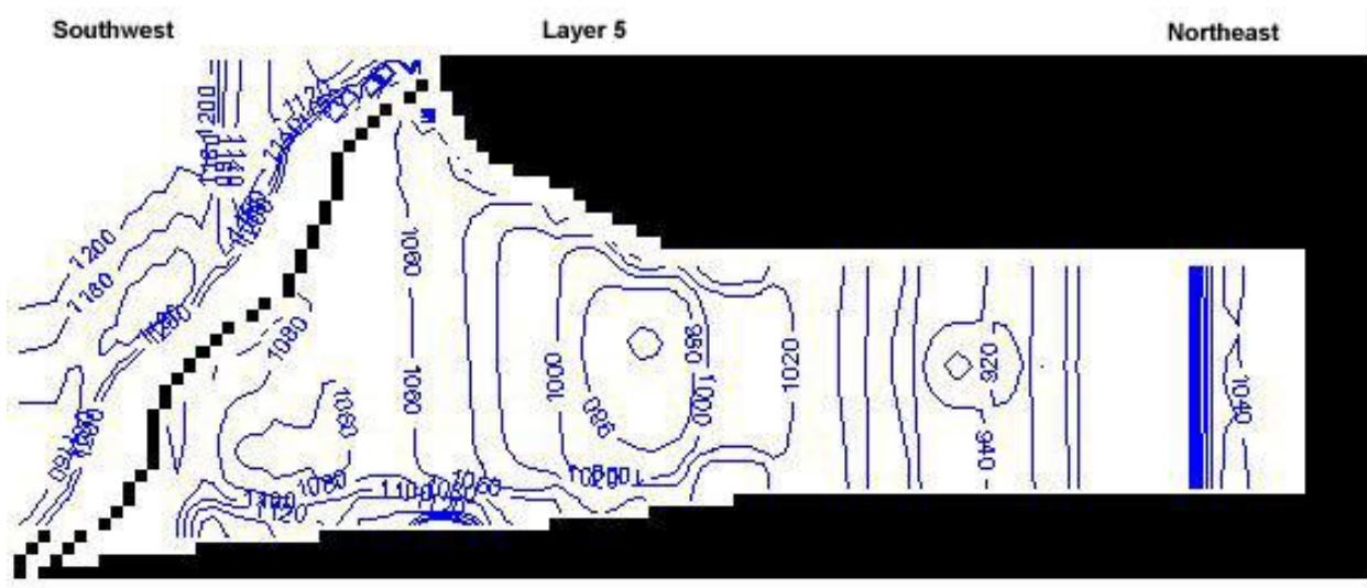
Figure 2. Potentiometric map of the Pittsburgh coal seam in the Irwin basin in the Groundwater Vista model. Contour interval is 20 ft.
