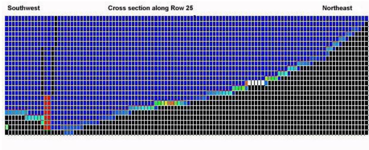
Figure 3. Color flood image of velocity along the longitudinal profile of the Irwin Basin Groundwater Vistas model. Velocities (ft/day): White >20; Red 18-20; Orange 16-18; Yellow 14-16; Lime-green 9-14; Aqua 4-7; Dark Blue 0-3.
