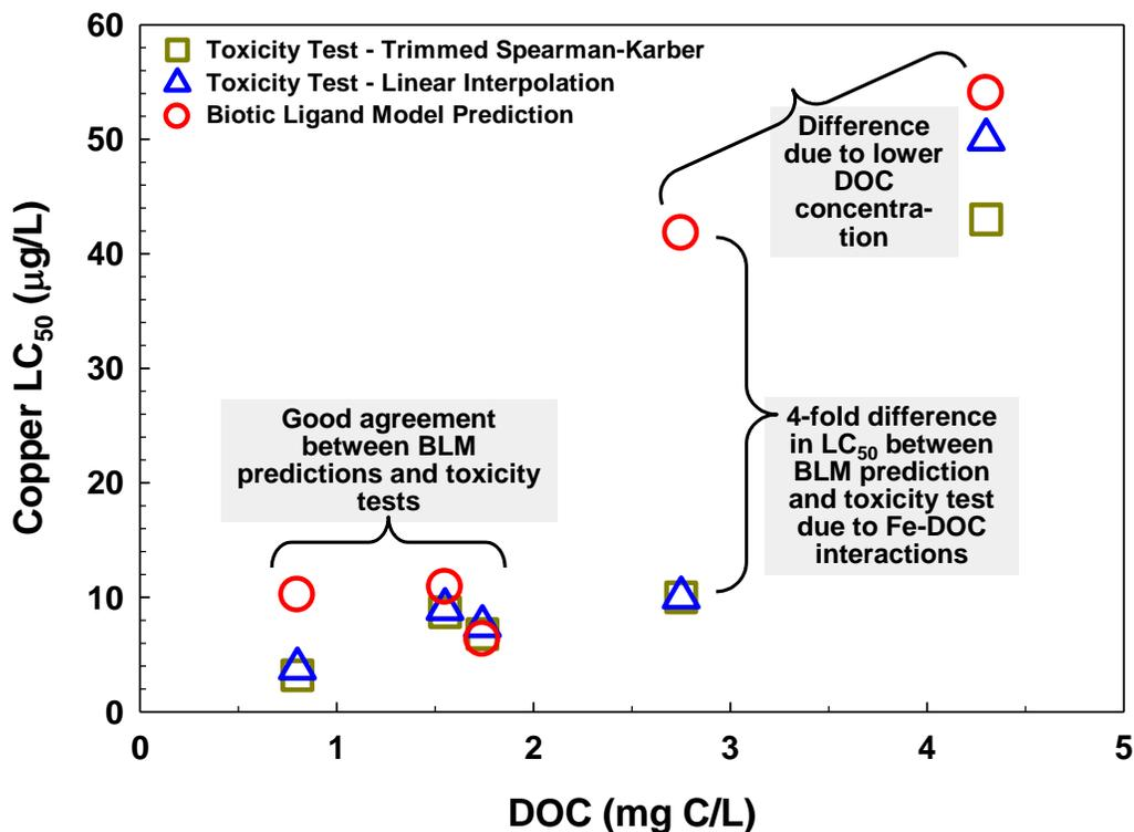
Figure 7. Comparison of Cu LC<sub>50</sub> values from traditional toxicity tests using *C. dubia* and from predictions computed by the BLM as a function of dissolved organic carbon. Approximately 2 mg/L Fe was added to selected test solutions. Test solutions are based on stream-water samples from drainage basins underlain by plutonic rock.
