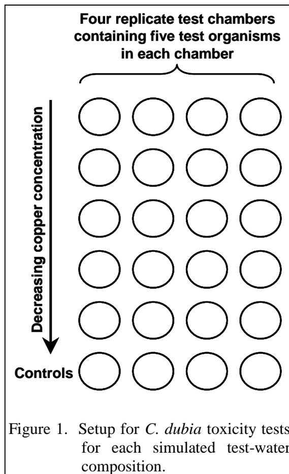
Figure 1. Setup for *C. dubia* toxicity tests for each simulated test-water composition.
