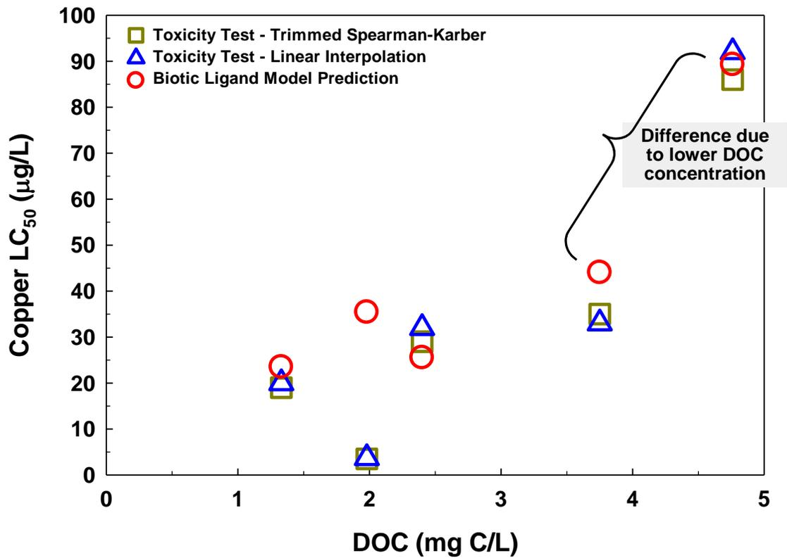
Figure 8. Comparison of Cu LC<sub>50</sub> values from traditional toxicity tests using *C. dubia* and from predictions computed by the BLM as a function of dissolved organic carbon. Approximately 0.5 mg/L Fe was added to selected test solutions. Test solutions are based on stream-water samples from drainage basins underlain by sedimentary rock.
