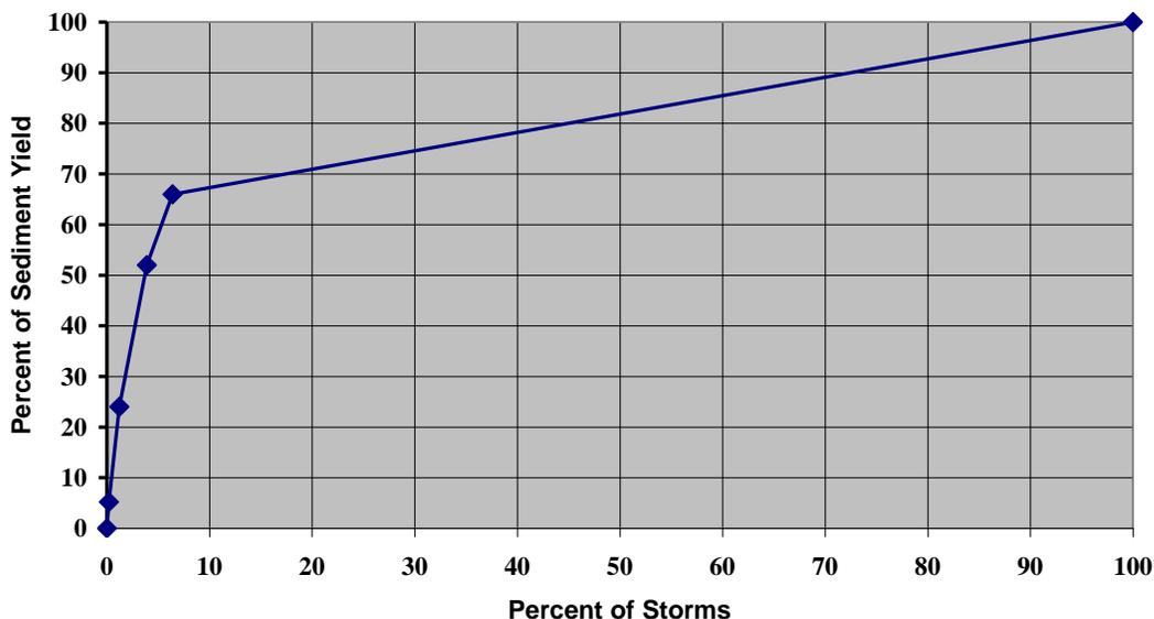
Figure 1. Illustration of the relationship between storm size and sediment yield on the erosion plots at Kingdom City, MO.
