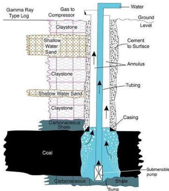
Figure 2: Typical Design of Coalbed Methane Well (Wyoming State Engineers Office).
