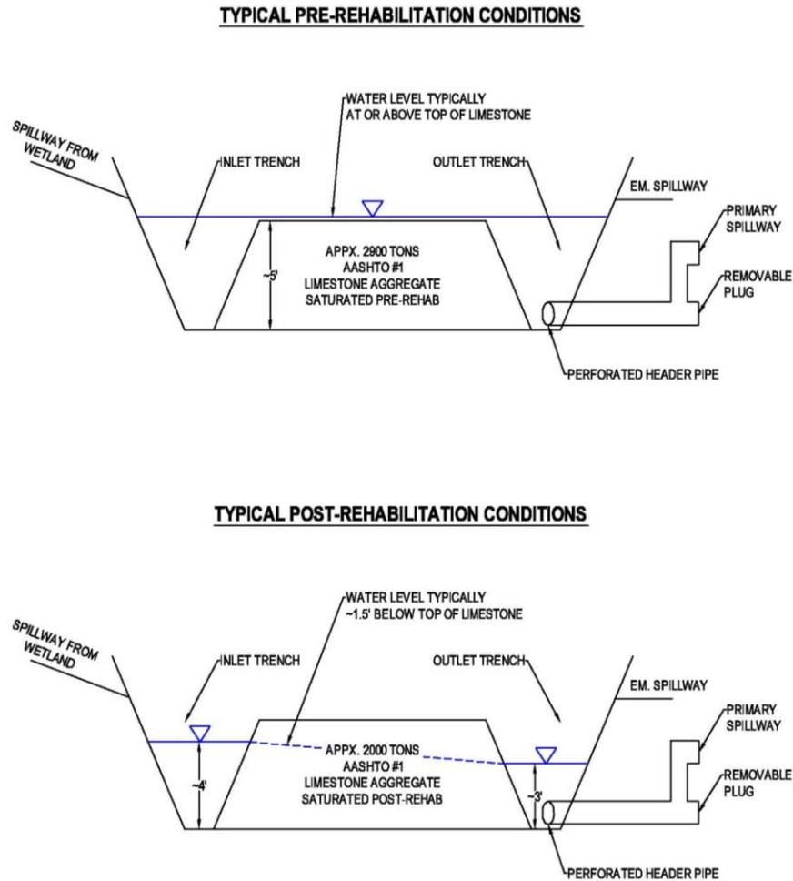
Figure 7. Typical Pre- and Post-Rehabilitation Conditions of the HFLB
