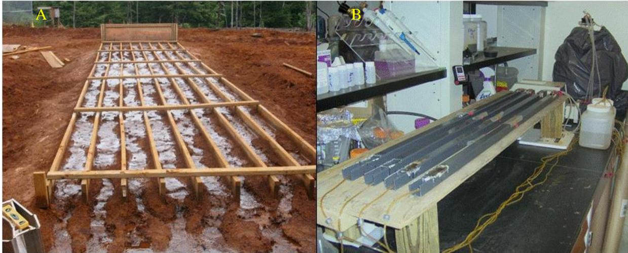
Figure 3. A) Picture of the channel reactors built on the Hughes Borehole iron mound. B) Picture of laboratory-scale “gutter” reactors showing the feed tank in the background and the four open-channel, flow-through reactors in the foreground.
