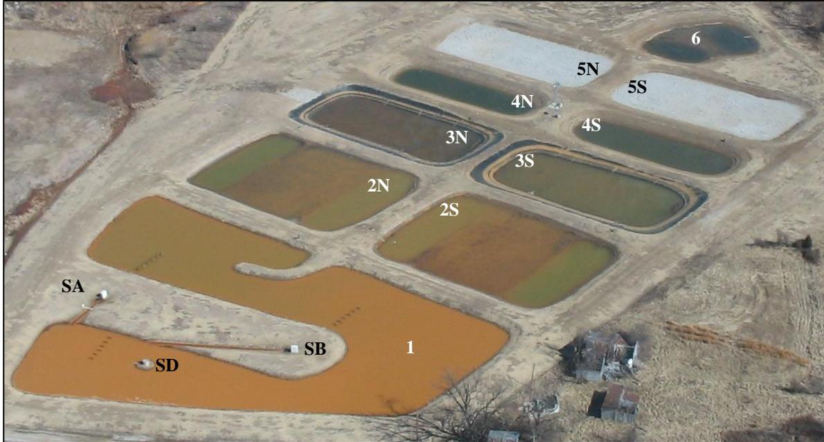
Figure 2. Oblique aerial photograph of passive treatment system taken February 4, 2009 showing mine drainage discharges and individual process unit designations.
