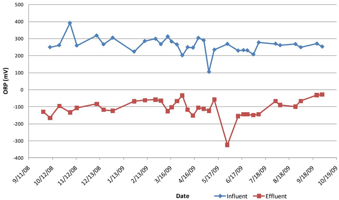
Figure 2. Pilot oxidation reduction potential values.
